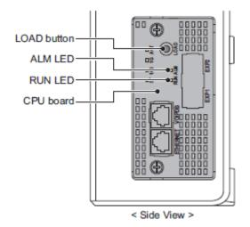
Also referred to as '**COLD Start**' can also be used at any time to delete the customer's configuration. Warning – COLD Start should only be used when you want to delete the customer's configuration from the SL2100 CPU card.
