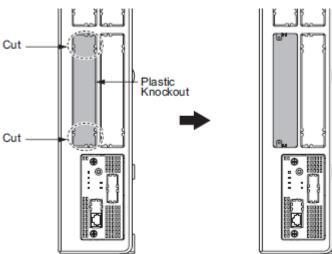
Note – the knockout can not be replaced once removed; there are no blanking covers available, be sure to remove the correct knockout.
